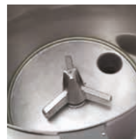
Residual water drain
